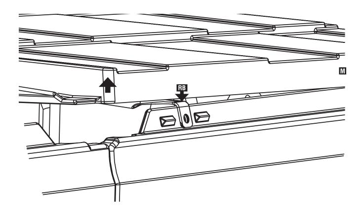
Ensure Repeat Roof (M) is positioned against the back wall tongues.
